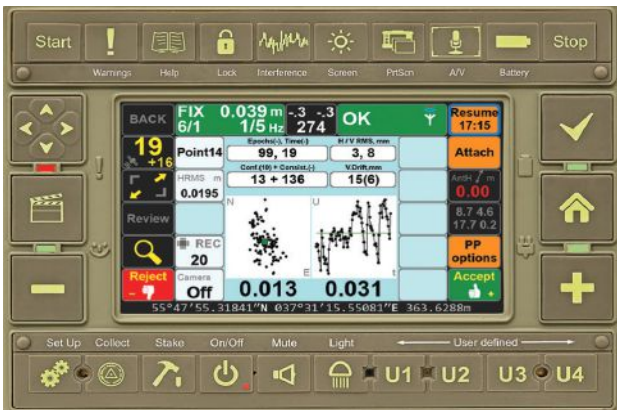
Status of RTK survey collection.
