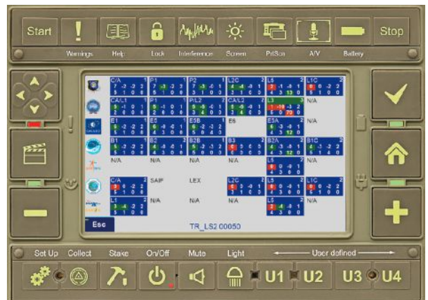
FIGURE 6. Signal Status. Information on all GNSS signals received as shown by the Triumph-LS.
