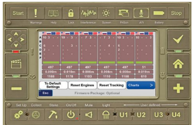
Six parallel RTK engines.
