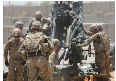
L3HARRIS DEVELOPS gun-hardened anti-jam solutions for the M1156 Precision Guidance Kit Modernization program. The kit turns 155-mm artillery shells into smart weapons. Here, soldiers test the kit for accuracy.
