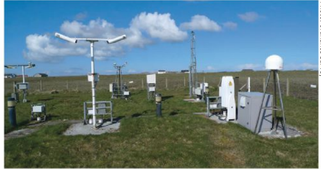
OS NET STATION: A CORS station in Tiree, the Hebrides, part of the Ordnance Survey's 110-strong OS Net network.
